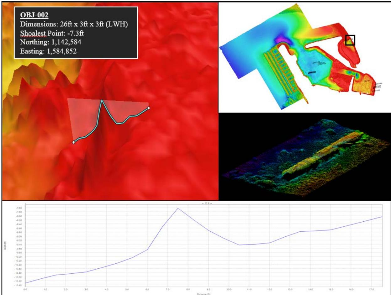
**Figure 40 OBJ-002: 3D, Profile, Point Cloud, and Overview**
