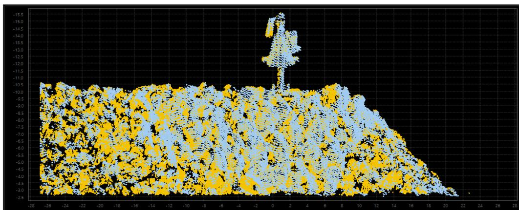
**Figure 11 Example Post-Boresight Calibration**
