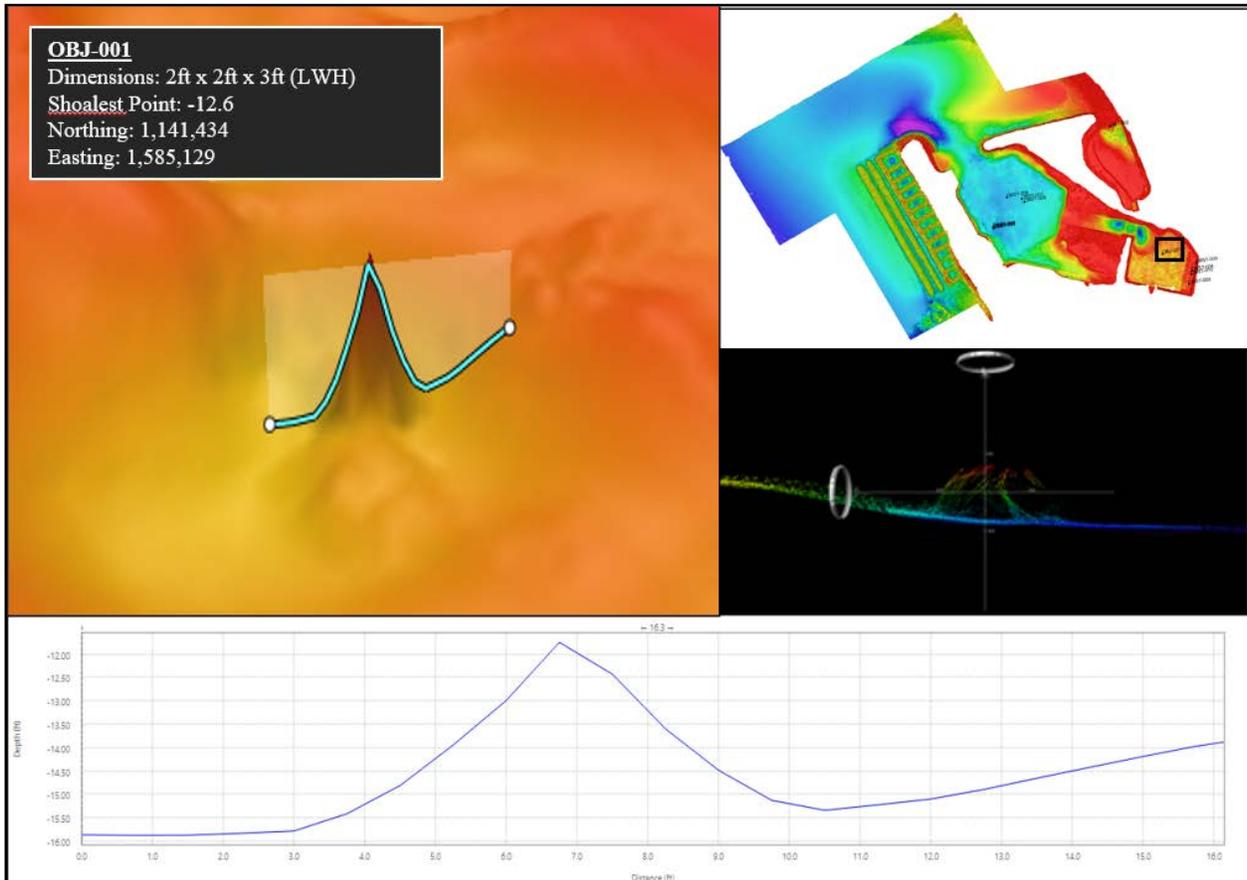
**Figure 39 OBJ-001: 3D, Profile, Point Cloud, and Overview**
